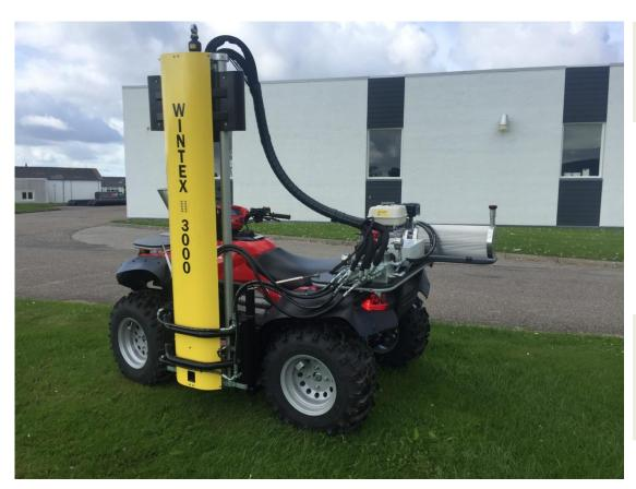
The WINTEX 3000 is an efficient and strong fully automatic soil sampler. It is user-friendly, easy to use and requires only minimum maintenance. All functions are comfortably carried out from the driver's seat.
